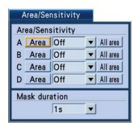
Up to 4 detection areas (A - D) can be set. It is also possible to set the whole displayed area as the detection area by pressing the [SET] button after moving the cursor onto the [All Area] button.
