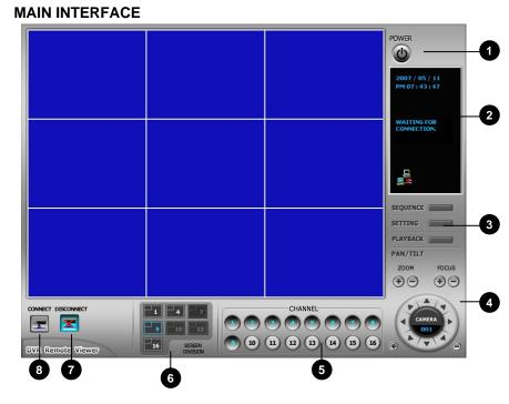
• Power button : Press the Power switch to exit the program. Please disconnect the live feed before powering off the software
