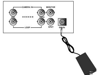
Connect one DC 12V, 6.67 A Adaptor to the back side of Power Jack for right operation of 2HDDs and CD Recorder.
