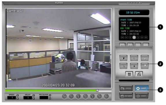
1. **RECORDED DATA DISPLAY :** Displays start time & end time of recorded data. Also, displays operating status during playback.
