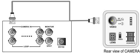
Connect cameras to the camera input on rear panel of DVR marked CAMERA IN.
