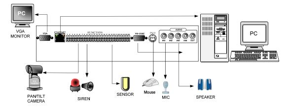
RS-232C : Control DVR through RS-232C port by using PC. RS-485 : Control external device like PTZ Camera RELAY Output : Relay Output – Pin No.4 ~ No.6 at Terminal Block SENSOR Input : SENSOR Input (Alarm connection) – Pin No.7 ~ No.26 at Terminal Block ETHERNET : Connection to LAN, WAN, Internet. VGA : Connection to a VGA monitor(CRT,TFT LCD) if optional VGA board is fixed
