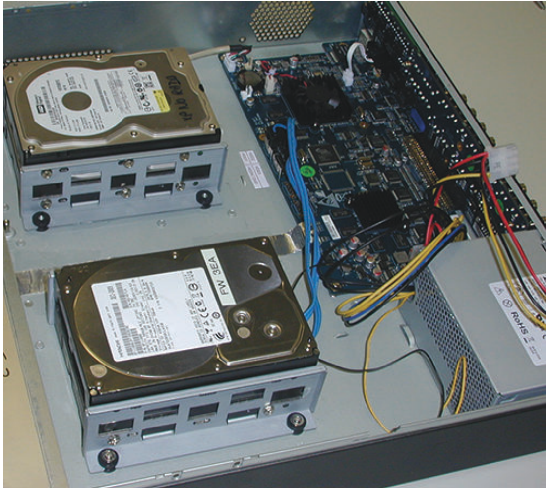
Figure 11.10: Install HDD 3 and 4
